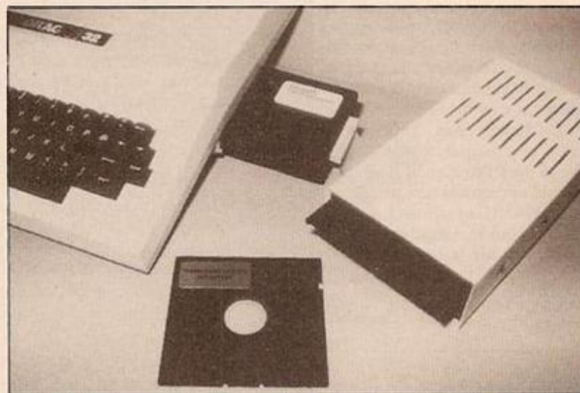
This includes the controller, cables, and a 40-track Canon disc drive with a capacity of 100K.
